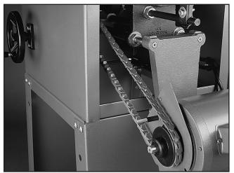
Figure 40. G3640 Power Twist® V-Belt installed.
